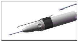
Insert the tubing end onto the proximal rod end of the spray clip.
