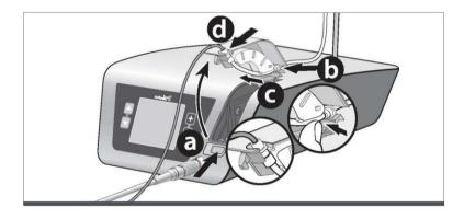
a Open the pump arm doorb,c Insert the irrigation pump tubingd Close the pump arm door
