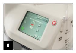
Touch "Disposable set is loaded" button. Select the desired processing protocol and change the whole blood volume if necessary.
