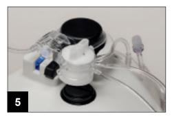
Place the pump loop tubing over the pump rotor. The pump loop will automatically load when the processing cycle is initiated.
