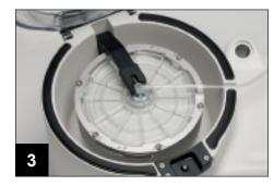
Once aligned, press down and turn clockwise until the position indicators snap into place. Lower the centrifuge stator arm and align it with the raised tab on top of the separation chamber.
