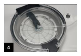
Place the tube leading from the separation chamber through the centrifuge well slot. Close the centrifuge lid.
