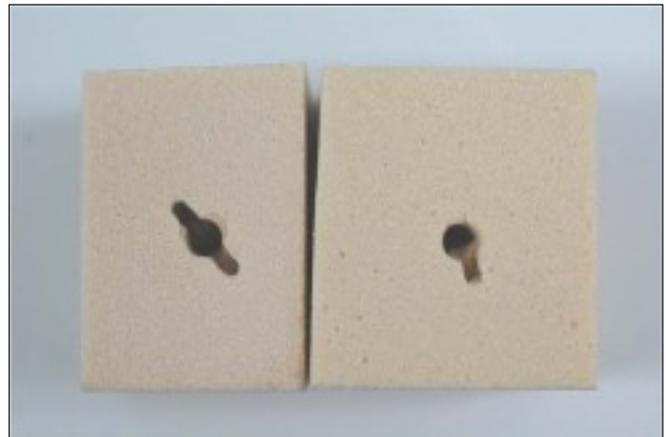
Porcine bone models are used extensively in biomechanical testing of ACL graft fixation devices because the biomechanical properties of this kind of bone tend to be more consistently superior to those of cadaver bones. The three samples of the ZipLoop all pulled through the cortical layer of the porcine bone at a mean load of 655N. The load required to pull the same button through the cortical layer of a human femur may be even lower.
