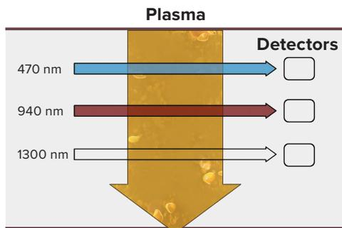
When plasma is present, all 3 light beams pass through and contact the detector. The Angel device recognizes the presence of plasma and turns the valve to collect PPP. The PPP is deposited in the PPP collection reservoir.
