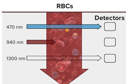
The 940 nm wavelength is absorbed by RBCs. When the detector no longer detects the 940 nm beam, the Angel system will allow a percentage of RBCs to pass through into the PRP collection syringe. The percentage of RBCs collected in the PRP syringe is determined by the hematocrit (HCT) setting selected by the operator.
