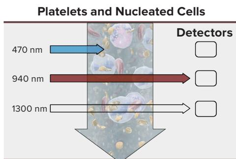
When platelets and nucleated cells are present, the 470 nm wavelength of light is absorbed. The absence of the 470 nm beam on the detector alerts the Angel system to stop collecting PPP. The Angel system will then actuate the valve to collect PRP. The PRP is directed into the collection syringe on top of the unit.
