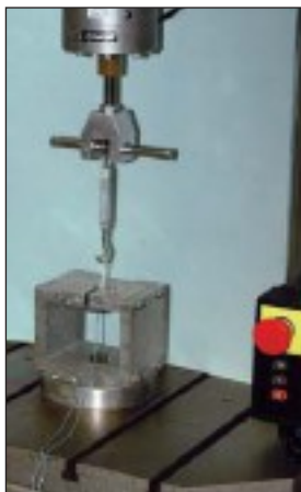
Figure 1: A 50 mm RetroButton secured in an Instron materials testing machine
