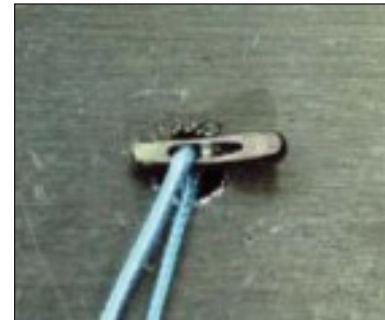
Figure 2: The suture loop is fed through a 4.5 mm diameter hole drilled through the steel plate
