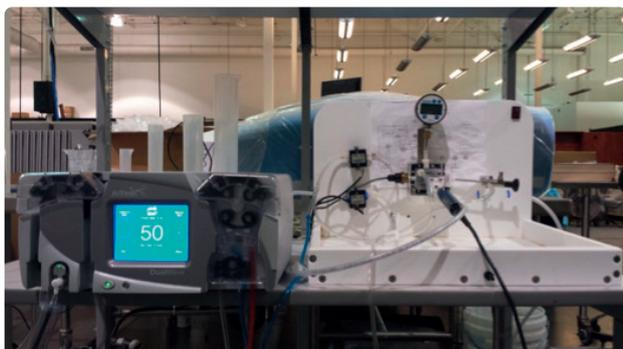
Using onboard fluid usage monitoring capabilities, the DualWave arthroscopy pump measured the total fluid used. This system provides real-time data on the fluid rate while running and displays the total fluid used when stopped. The arthroscopy pump was turned off between each test to fully reset the fluid usage monitor.
