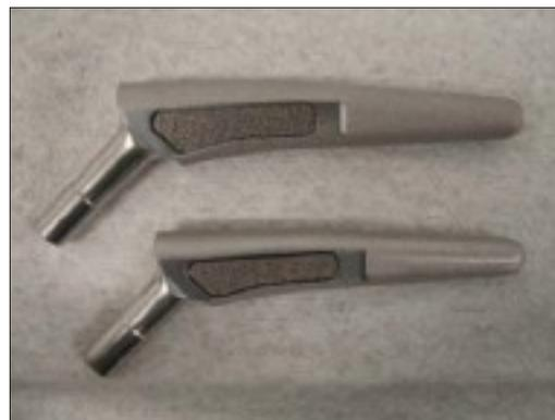
*The device for the canine total hip study. Clinically available canine hip stems (BioMedtrix BFX) were modified to remove the standard sintered beaded coating and replace it with BioSync pads on the anterior and posterior surfaces in the proximal region of the stem.*
