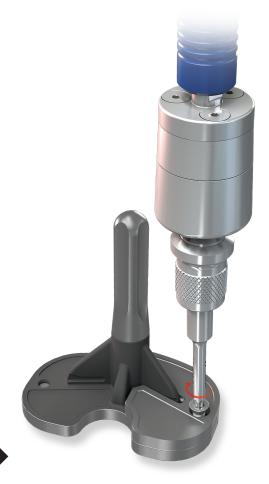
Tighten the included augment screw to 3-4 Nm using the torque indicating driver.
