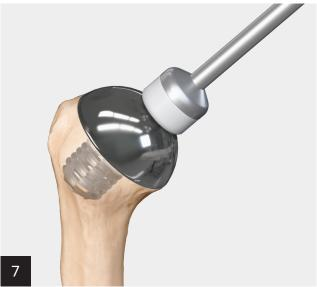
Select the appropriate humeral head and impact the humeral head onto the trunnion using the head impactor.
