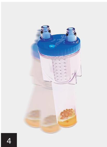
Shake the device for 5 seconds to break the clot.
