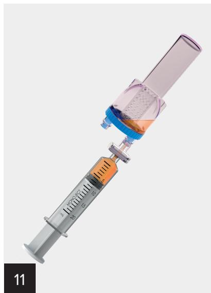
Connect the filter to the “withdraw” port. Invert the device at a 45° angle toward the “withdraw” port and withdraw serum through the filter.
