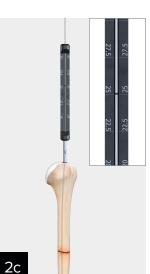
Use the guidewiremeasuring gauge and black line on the guidewire to determine the length of the humeral nail needed.
