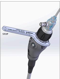
**To tighten the scope on the head:** Screw the scope on to the Synergy<sup>UHD4™</sup> C-mount camera head by hand until tight. Place the wrench on the silver nut **(A)** on the scope. While holding the camera head firmly, **PUSH the wrench clockwise** to tighten the scope on the camera head.
