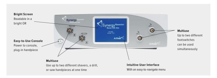
This versatile Synergy<sup>Resection</sup> system was designed for multiple arthroscopic procedures and operates like two consoles in one chassis. It can simultaneously operate two accessory handpieces completely independent of each other. Operators can also use one or two foot pedals to control each of the accessory handpieces. Shaver handpieces offer three oscillating modes depending on the application or surgeon's preference: standard, efficient, or aggressive.
