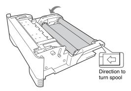
4 Set the selector for the paper holder (blue). Turn the knob on the paper holder (blue) selector to match the size of the paper roll.
