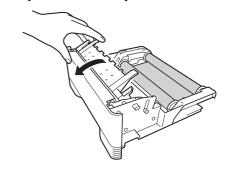
② Place the paper roll in the media tray so that the arrow on the label points toward the ink ribbon side. You can load the paper roll in the correct direction by matching the colors of the paper holders inserted into the paper roll with the colors on the media tray.
