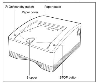
Press the printer ( On/standby switch to turn on the power of the printer.
