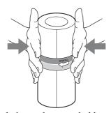
• Correctly insert the paper holders all the way.
