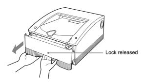
The media tray is normally locked in place when it is in the printer. The lever that releases the media tray is located behind the bottom edge of the tray. To unlock the tray, simply pull the lever with your fingers.
