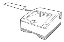
Press and hold the STOP button, and release the button when the CLEANING indicator flashes. About 20 cm of paper is fed out of the printer from the paper outlet.
