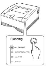
When cleaning finishes, the paper is ejected and the CLEANING indicator remains lit.
