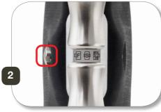
Forward-only mode. F Reverse will not operate. Depress bottom trigger to run the device in forward.
