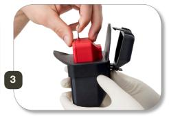
Align the rails of the battery and battery housing and push the unsterile, fully charged battery as far as it will go into the battery housing. Ensure the metal tab on the battery lays flat.
