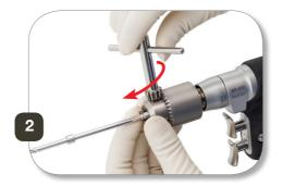
Fix the drill bit in the drilling chuck and tighten the connection until secure.
