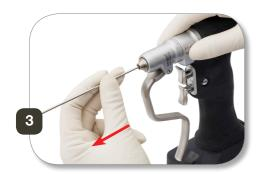
TIP: Lever pulled = wire not fixed. Lever not pulled = wire fixed.
