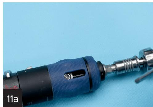
Hold tension on the cable as you feed it through the hole. Like the previous side, the cable should be visible in the set screw window. Use the driver to tighten the set screw until you hear 3 clicks.
