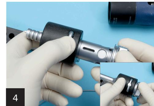
4 Press the bowtie button to click the metal connecting piece into place. The arrow/#3 should align with the bowtie button.
