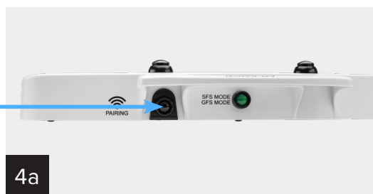
4 Pairing button - Pair footswitch by simultaneously pressing the receiver and footswitch pairing buttons, then release (footswitch must be within 6 feet of the receiver during this process). Note: The footswitch must be held vertically so that the handle is facing the ceiling when pressing the pairing button.
