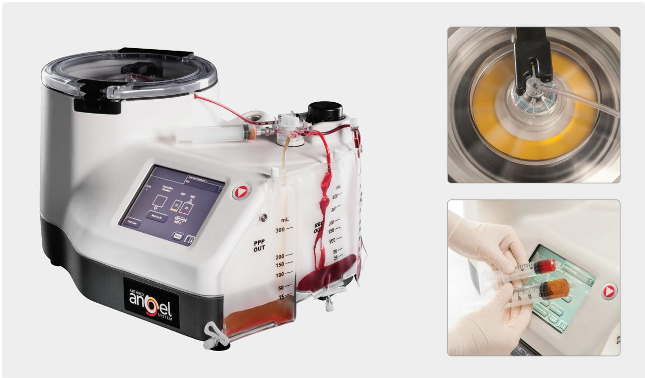
The Angel cPRP system is the only fully automated system that utilizes 3-sensor technology (3ST) and one-button automation to prepare customized formulations of PRP from whole blood or bone marrow aspirate (BMA). It can deliver platelet concentrations up to 18× over baseline with adjustable leukocyte concentrations.
