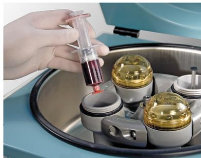
Centrifuge for 5 minutes at 1500 rpm.
