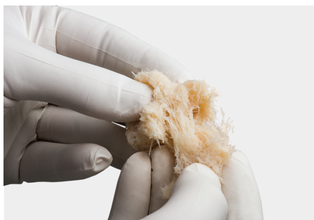
Entangled fibers create a 3D interconnected matrix to promote cell migration and fusion.
