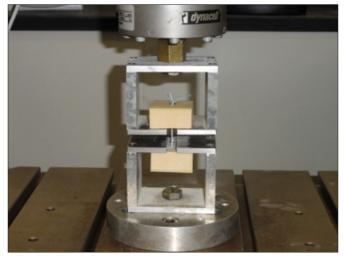
Test fixture for cyclic tensile test and load to failure
