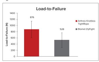
Load-to-failure of the TightRope and ZipTight in tension
