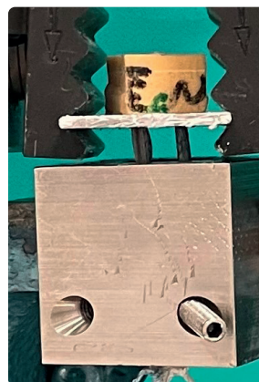
Figure 1A. Test setup with bone blocks and cerclage.
