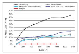
Percent Mass Loss  $\%\Delta m$  as a function of applied load. Data points for materials other than BioSync were taken from a graph in the literature and are estimated to be accurate to  $\pm 1\%$ .<sup>20</sup> At all loads tested, BioSync structure abrasion was negligible and significantly lower than that for the other porous scaffolds.
