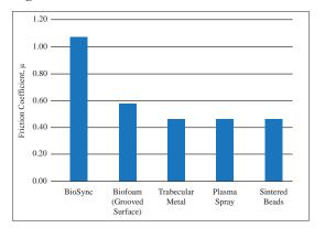
Friction coefficient of bone ingrowth materials tested against 10 pcf SAWBONE. Results for materials other than BioSync structure were taken from Brownhill.<sup>18</sup>
