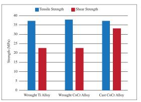
Static strengths of BioSync structure when combined with various metal substrates. Due to fixture failure rather than sample failure during some of these tests, these reported strengths are lower than the actual sample strengths. Even so, all strengths satisfied FDA requirements.
