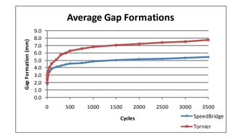
The mechanism of displacement for the Tornier samples was always sutures cutting through the bone tunnels, as shown in Figure 3. On average, the amount of bone cut by the sutures was  $6 \pm 2$  mm. Conversely, the knotless SpeedBridge repair did not show a tendency for the FiberTape to cut through the bone and moves the mode of failure from the bone to the tendon.
