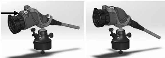
Figure 2: Installing camera into snap-fit Camera Mount
