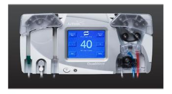
Effective outflow control provides a clear, consistent turbulent-free joint space for optimized distention and clarity.
