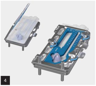
Ensure proper alignment of the mold in the base. Press and screw the base closed tightly.
