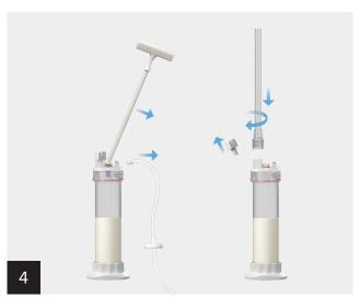
Pull the plunger up completely so that a blue line is visible, and snap off the plunger rod. Attach the nozzle and trim as desired based on the mold size.
