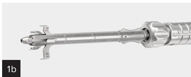
Starting with the “A” slot, select the leg with the length corresponding to the targeter leg length from the VIP™ preoperative plan (a), and load it into the slot labeled “A” on the targeter shaft until the end of the leg passes under the locking nut and meets a positive stop. Repeat this step for legs labeled “B” through “E,” matching them with the corresponding letters on the targeter shaft.
