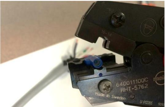
Place the Molex quick disconnects into the enclosed Molex crimping tool as shown.
