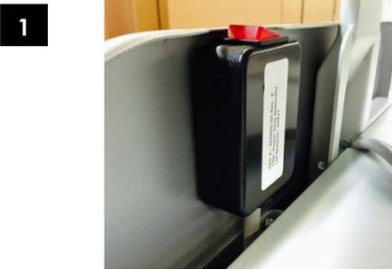
Remove remote switch box assembly from the cart. The remote switch is secured to the cart with double sided 3M VHB tape.
