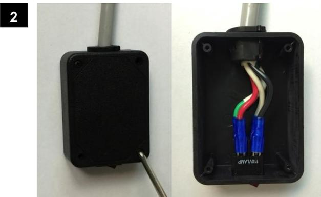
Remove the top cover plate of the plastic enclosure by removing the four corner screws with the enclosed #1 Philips-headscrewdriver.
