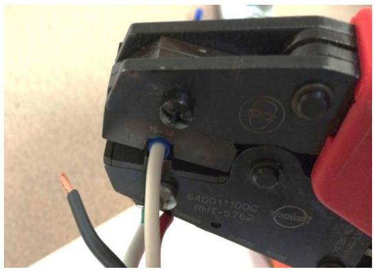
Insert the wire into the quick disconnects; fully seat the wire and crimp.
