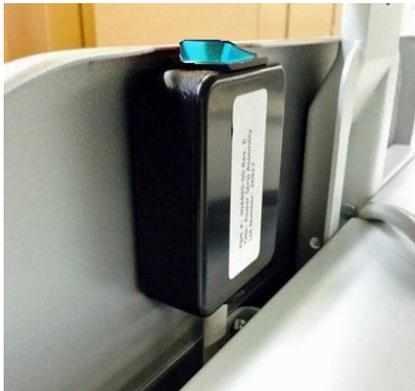
Install remote switch box assembly onto the cart from where it was originally removed. Peel off the paper of the 3M VHB tape and secure remote switch assembly to the cart.
