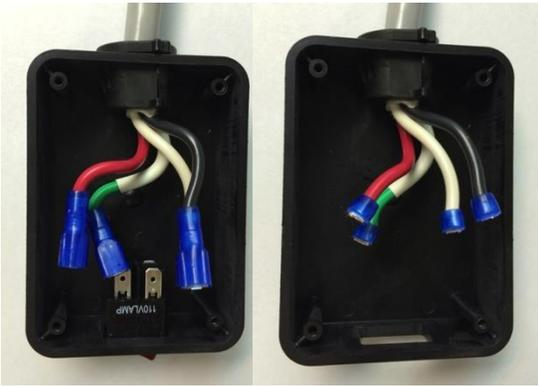
Disconnect the QTY (4) quick disconnects of the switch terminals. Cut the quick disconnects (blue connectors) as shown.
