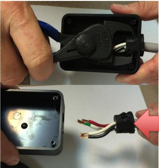
Remove the black strain relief with the enclosed strain relief pliers. Depress the tabs on the strain relief and remove the cable assembly from the plastic housing.
