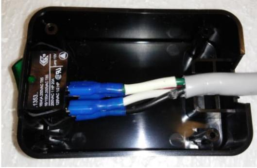
In the new switch case supplied with the kit, place the switch with markings facing up (as shown) into the cutout of the enclosure. Verify cord is placed on enclosure strain relief (as shown).
