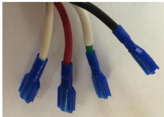
Crimp all QTY (4) wires. Finished assembly shown; quick disconnects crimped to each wire.
