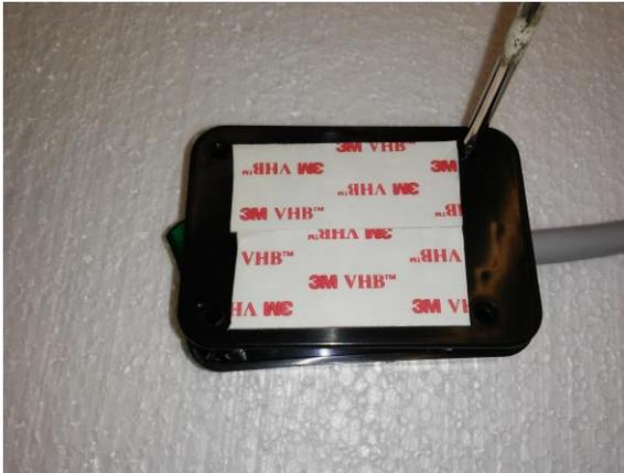
Place cover of the switch case and insert four corner screws. The replacement remote switch enclosure has the double sided 3M VHB tape preattached.
