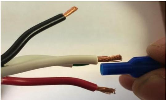
Make sure that there is 1/4 in of exposed wire; strip wire jacket with enclosed wire strippers if necessary.
