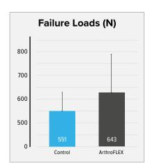
Comparison of failure loads (N) of human dermal allograft extracellular matrix augmentation vs control.
