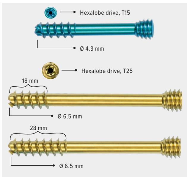
The cannulated titanium 4.3 mm and 6.5 mm headless compression PT screws can be used for fixation of osteotomies, fusions, and fractures in the midfoot and hindfoot. The headless design helps reduce the risk of profile complications, provides compression, and allows for simplified insertion.
