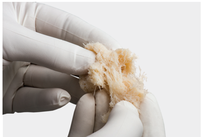
Entangled fibers create a 3D interconnected matrix to promote cell migration and fusion.
