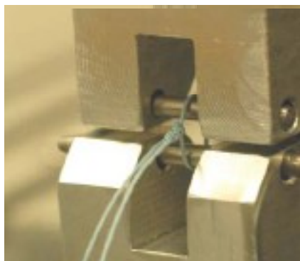
Figure 1. Knot Security Test Set-up
