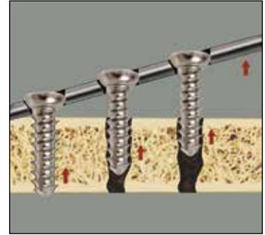
Bending load requires only screw pull-out to fail
