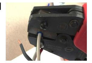
Insert the wire into the quick disconnects; fully seat the wire and crimp.
