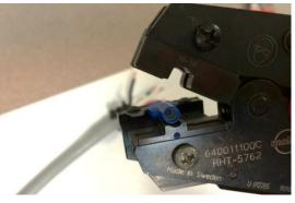
Place the Molex quick disconnects into the enclosed Molex crimping tool as shown.
