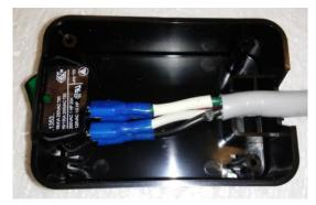
In the new switch case supplied with the kit, place the switch with markings facing up (as shown) into the cutout of the enclosure. Verify cord is placed on enclosure strain relief (as shown).
