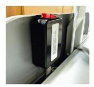
Remove remote switch box assembly from the cart. The remote switch is secured to the cart with double sided 3M VHB tape.
