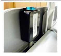
Install remote switch box assembly onto the cart from where it was originally removed. Peel off the paper of the 3M VHB tape and secure remote switch assembly to the cart.
