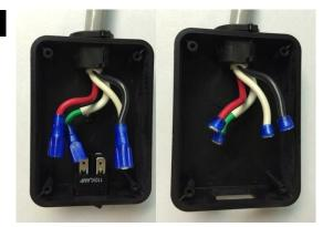
Disconnect the QTY (4) quick disconnects of the switch terminals. Cut the quick disconnects (blue connectors) as shown.
