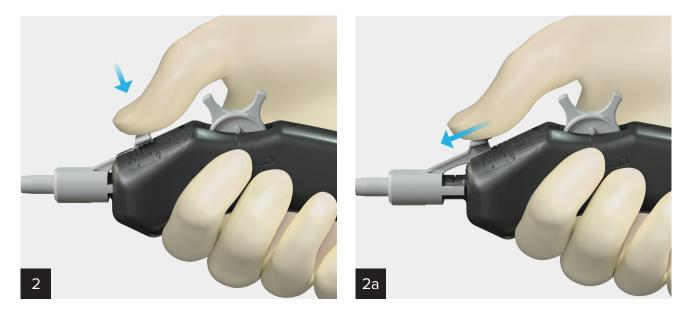
The depth stop is set to 18 mm. To change the depth stop setting, engage the selector by depressing the gray tab (2) and then advancing it forward to the desired depth setting (2a).
