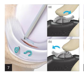
Deploy the second implant by rolling the deployment wheel backward to a hard stop and an audible click is heard. The deployment wheel will display a solid vertical indicator (a). Before removing the device from the tissue, roll the wheel completely forward to a hard stop (b).
