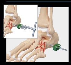
Place the first pin then slide the multipin clamp over it. Place the second pin through the clamp for two-pin fixation in the calcaneus. Set the clamp using the smaller T-handle.
