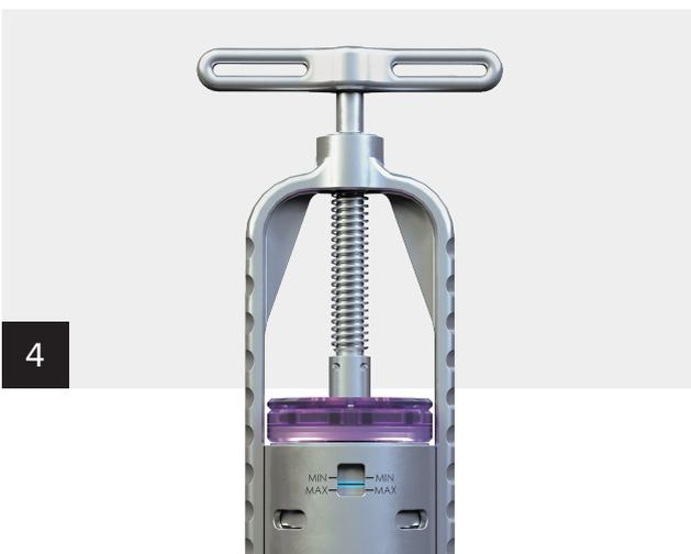
Load the plates onto the press and twist to lock in place. Turn the press handle clockwise until the indicator line is close to MAX. Allow a minimum of 4 minutes of compression before removing the plates.
