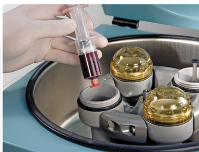
Centrifuge for 5 minutes at 1500 rpm.
