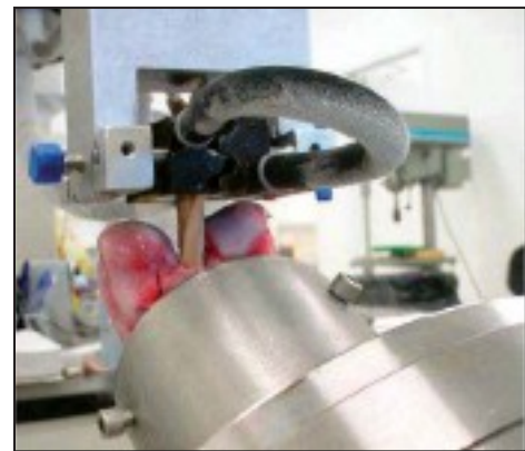
Figure 2: Repaired tendon fixed in the Instron System for testing
