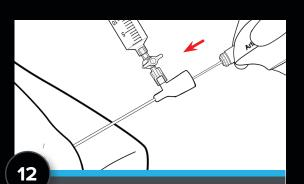
Insert NanoScope handpiece hypotube into cannula and lock into place.
