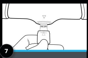
Insert connector end of handpiece into NanoScope console until fully seated.
