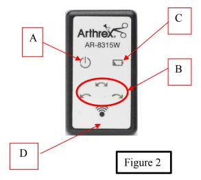
3. To begin the footswitch and receiver pairing process, position the footswitch vertically and within six (6) feet (1.8288 meters) of the receiver during the entire pairing process.
