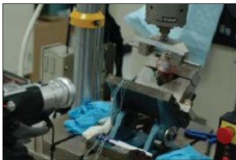
The graft was precycled from 10 to 50 N at 1 Hz for 10 cycles, followed by cycling from 50 to 250 N at 1 Hz for 500 cycles. Post-cycling, pull-to-failure was conducted at 20 mm/min.
