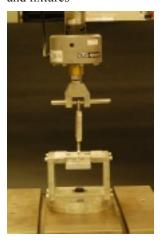
**Figure 2:** Suture link centered on hook fixture
