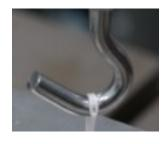
**Figure 4:** Suture link severely off-center
