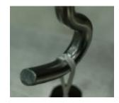
**Figure 3:** Suture link off-center on hook feature
