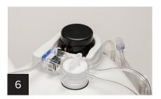
Press down firmly on the backside of the platelet cuvette until the assembly is snapped in place.
