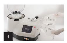
Remove the Angel cPRP processing set from the tray and place it on top of the machine.
