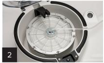
Insert the variable-volume separation chamber into the centrifuge adapter by aligning the notches.
