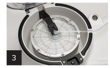
Once aligned, press down and turn clockwise until the position indicators snap into place. Place the tube leading from the separation chamber through the centrifuge well slot.
