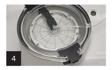
Lower the centrifuge stator arm and align it with the raised tab on top of the separation chamber. Close the centrifuge lid.
