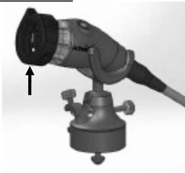
Figure 3: Removing camera from snap-fit Camera Mount
