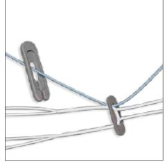
Align the Button Extender underneath the TightRope button in the orientation in which it will be passed. Begin by passing the inferior blue passing suture through the Button Extender.
