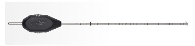
**FlipCutter**<sup>®</sup> **III Drill:** The innovative FlipCutter III drill is an adjustable, variable-size, all-in-one guide pin and reamer that allows minimally invasive socket creation from the inside out. The drill simplifies the technique and costs associated with quadriceps tendon grafts in which each end may be slightly different in size.
