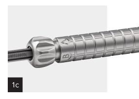
Slide the locking nut down the exposed shaft to meet the edge of the handle. Do not tighten the locking nut to allow adequate room for the targeter legs to slide in place between the shaft and locking nut.
