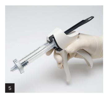
Rotate the collar to "inject." Insert the syringe into the gun with the markings on the syringe facing upward. Compress the trigger to push the piston forward and expel any excess air.
